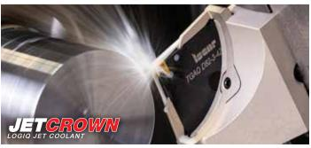
In pressure control machining parts, high-temperature alloys generate very high temperatures as they are being cut. By effectively removing metal with **JET-HP-LINE** products, which feature high-pressure coolant (HPC) supply, the cutting-edge tool life is dramatically improved, and the chips become less ductile and thus easier to break.
